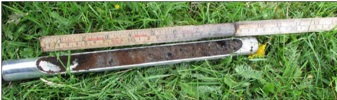
Fig. 50. A typical core from the ash pit area. Note the layers of brown soil between layers of ash.
