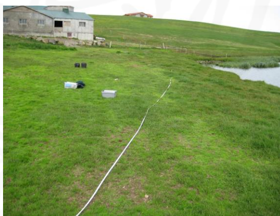
Fig. 11. Coring transect 2 ran 20 m roughly N-S, parallel to the lake shore. Looking NW.
